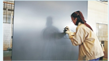
Appearance, coating thickness, gloss, colour different quality inspection
